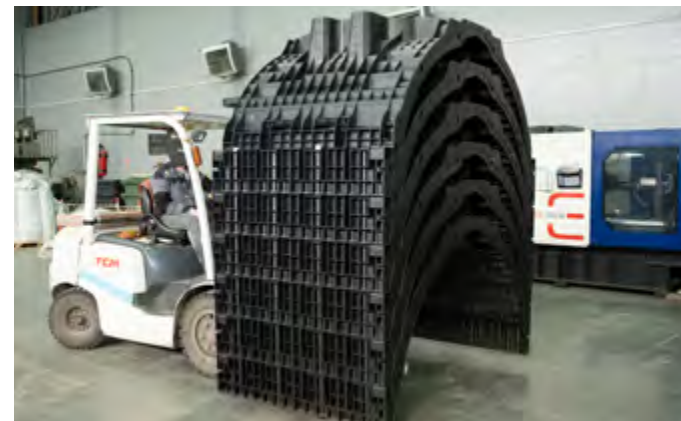
Loading of an "AQUABOX" Tank
