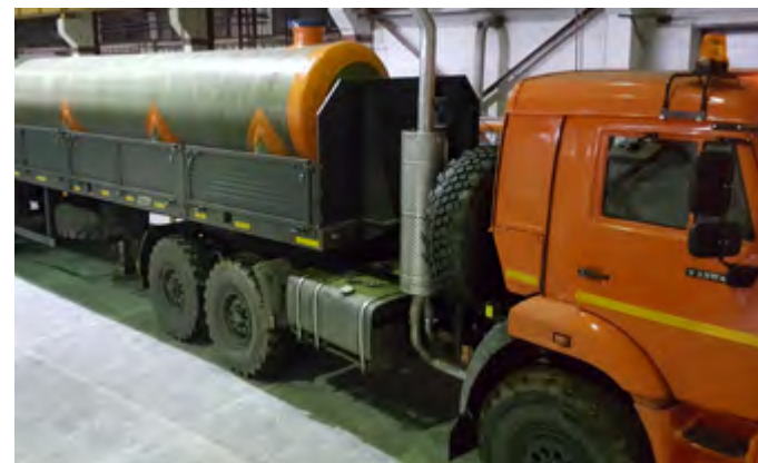
Transportation of a Fiberglass Tank
